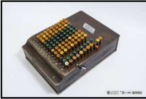
Felt & Tarrant Manufacturing Company Comptometer Model B (ca. 1915). Calculadora mecánica de tecla pulsada
